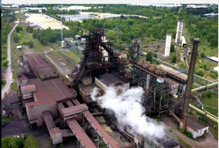
ArcelorMittal's project to inject natural gas into the H05A blast furnace in cooperation with N0PA aimed to improve the C02 balance. Significant C02 savings were achieved through the installation of a system for controlled natural gas injection. N0PA contributed to significant cost savings by optimizing valves and reducing pipe diameters and the number of valves.
